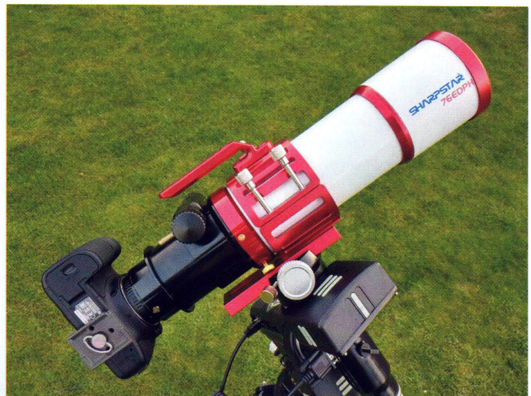
▼ The SharpStar 76EDPH plus f/4.5 reducer–flattener with a Canon 6D camera attached.
