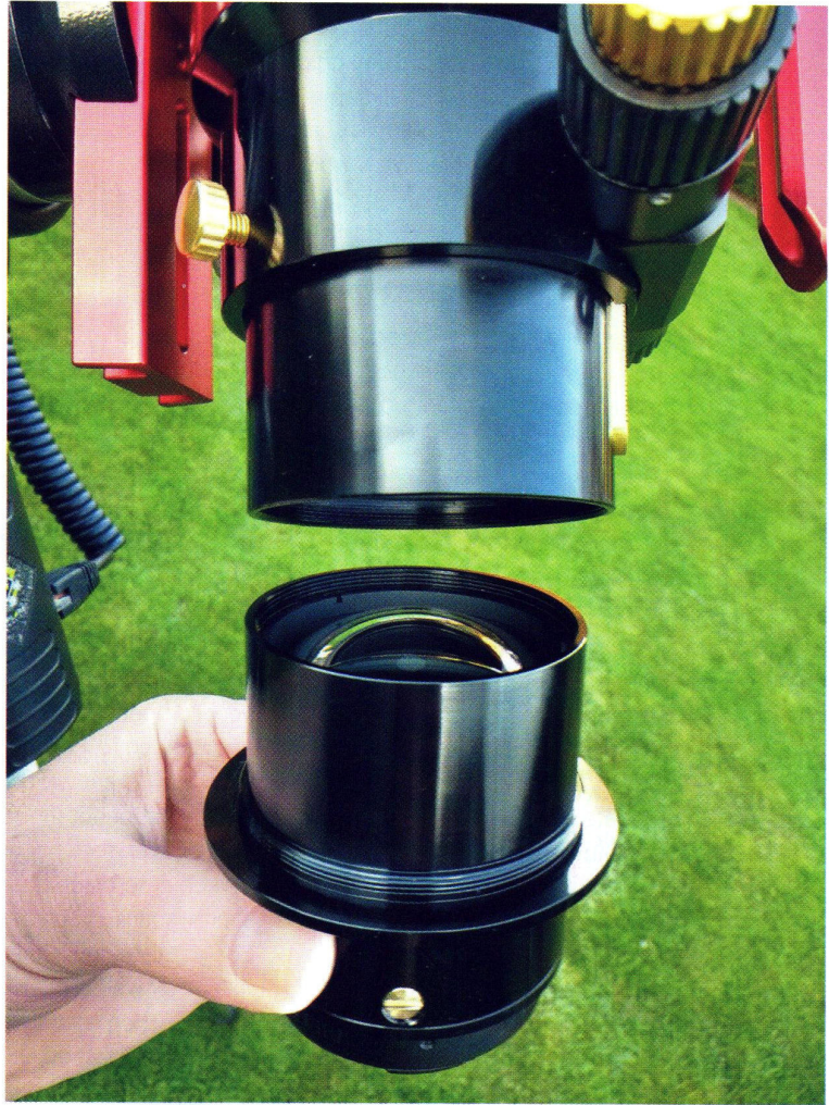
▲ Converting the 76EDPH from visual to 'astrographic' mode with the f/4.5 full-frame reducer–flattener entails unscrewing the drawtube's visual back, exposing a female M74 \times 1 thread, then screwing the nosepiece of the 77mm-long reducer in its place.
